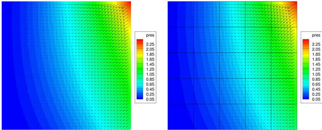
Fig. 2. Computed pressure (color) and velocity (arrows) in Example 1: fine scale solution (left) and multiscale solution with a single linear mortar per interface (right).
