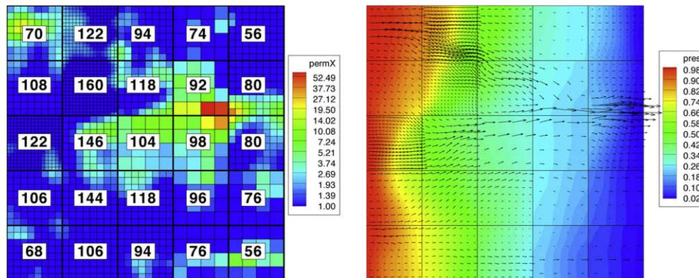
**Fig. 6.** Permeability field for Example 4 on mesh refinement level 4 (left) and its corresponding solution (right). Numbers indicate the total number of subdomain solves using the Multiscale Flux Basis implementation.
