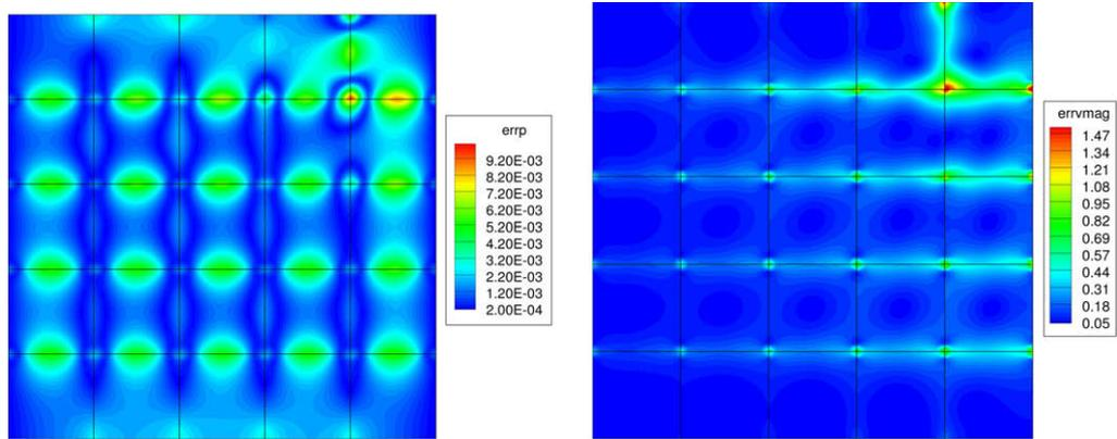
Fig. 3. Pressure error (left) and magnitude of velocity error (right) for the multiscale solution with a single linear mortar per interface in Example 1.
