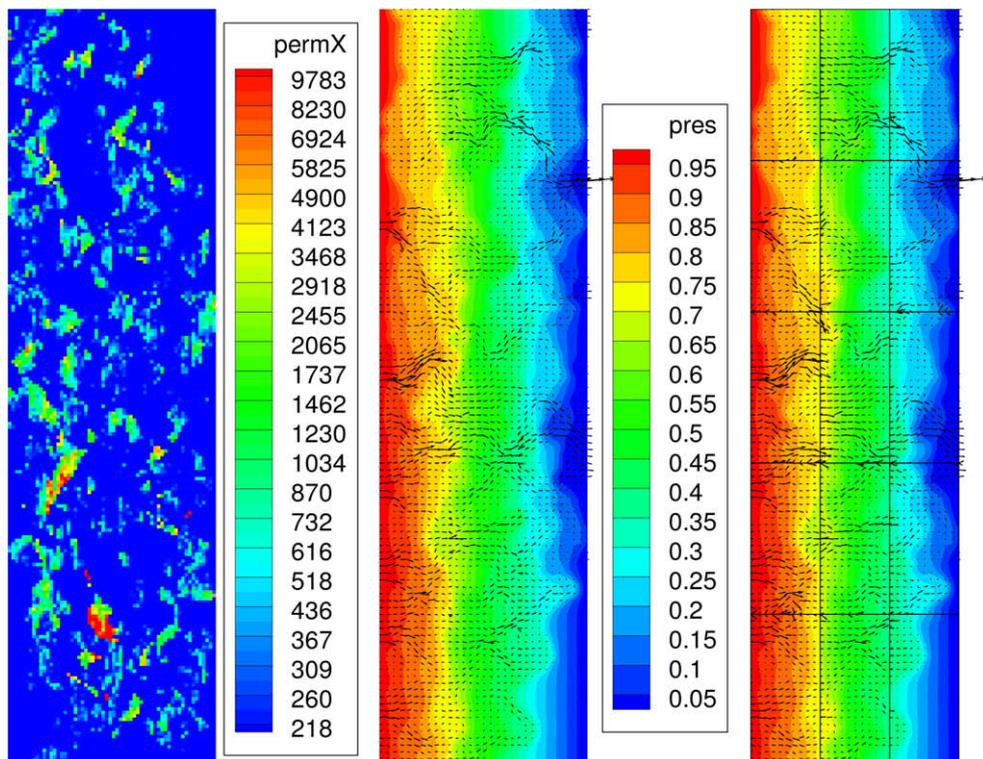
Fig. 4. Example 2: permeability field (left), fine scale solution (middle), and multiscale solution with  $3 \times 5$  subdomains and a single linear mortar per interface (right).
