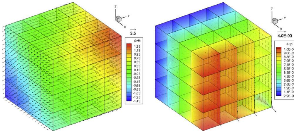
**Fig. 5.** Example 3: computed multiscale solution (left) and its error (right) on  $4 \times 4 \times 4$  subdomains with a single linear mortar per interface.
